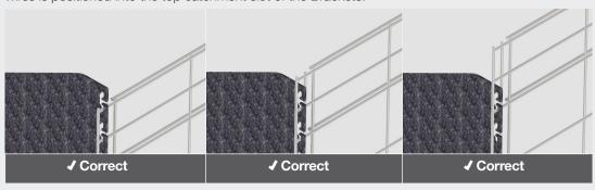
When inserting the Panel into the bottom Brackets, ensure that one of the three bottom-most horizontal wires is positioned into the bottom catchment slot of the Brackets.
