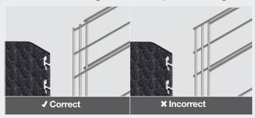
When inserting the Panel into the Brackets, ensure that the Bracket catchment slots are positioned between the three outermost vertical Panel wires.
